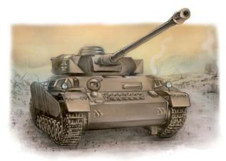
The bow machine gunner/radio operator uses a second MG34 in the body front and manages the radio (5-mile range). Many tanks have a *third* MG34 at the commander's
